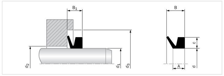
For pressures from 40 MPa to the maximum specified, use diameter tolerance H8/f8 (bore/rod) in the area behind the seal.
